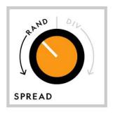
Turning SPREAD counter-clockwise from noon causes the "moons" to generate random patterns. The further counter-clockwise, the more quickly these patterns evolve. Turn SPREAD back to the noon position to lock the randomly-generated pattern.
