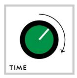
From noon to the full CW position, the TIME knob adjusts the delay time like a traditional analog-style delay effect. The farther CW the knob is turned, the longer the delay time.
