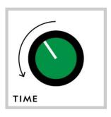
The glitch delay and reverb modes are accessible when the TIME knob is turned CCW from the noon position.
