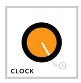
Pluto can be synced to an incoming sync signal or MIDI clock. To initiate sync to an external clock source, turn the CLOCK knob to the full CW position.
